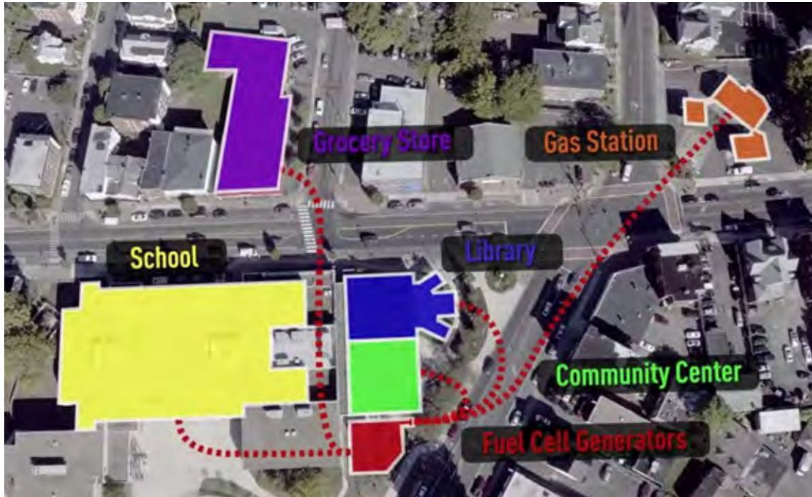
**Figure 16** ■ Diagram of microgrid operations during normal and emergency operations (Constellation Energy)
